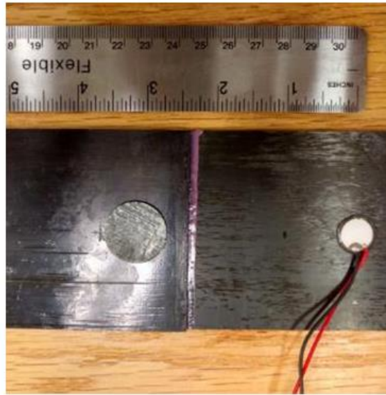
Figure 4.8 The simulated damage on the composite lap joint
