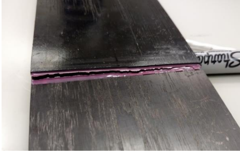
Figure 4.15 Catastrophic failure of the lap joint.
