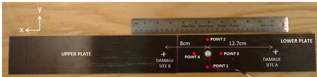
Figure 4.25 The sites of actual damage A and B.
